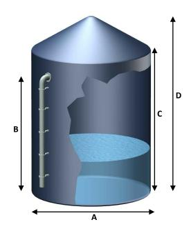
All measurements are based on tanks having 20 deg conical roof. Other tank volumes and sizes are available. List is shown as guidance only.
