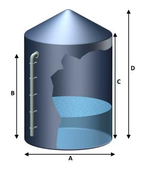
All measurements are based on tanks having 20 deg conical roof. Other tank volumes and sizes are available. List is shown as guidance only.
