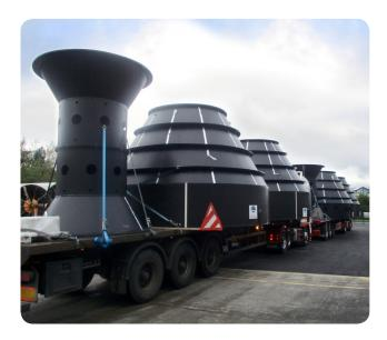
The 60° conical hopper slope allows even fine solids to be transported to the base of the tank for removal, assisting the production of a clarified effluent. The external structure of the tank cone is complete with reinforcing ribs which double as locating lugs to eliminate post installation movement of the tank in its surrounding media. The stiffening ribs incorporate drilled holes to allow the 'keying' of concrete.
